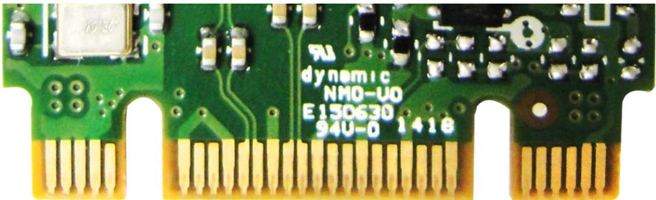
Figure 3 : The connectors of M.2 2242 SATA III SSD
