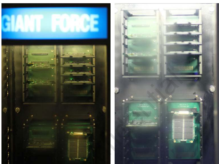
Figure 6: Memoright 1.8" PATA ZIF & 2.5" SATA SSD burn in
