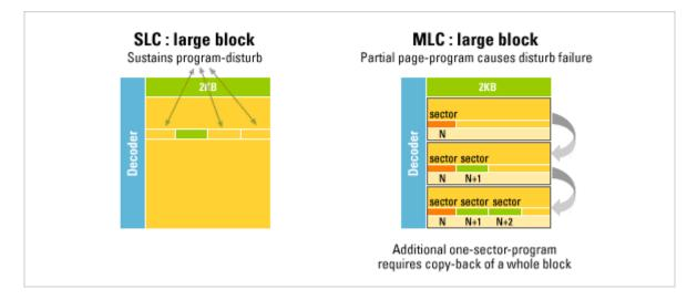
SLC NAND Flash optimizes information transfer and data flow, since all the pipes which are program-to-program communications, are the same. However, with MLC NAND Flash, the pipes are different and the information transfer and data flow can be uneven and slow.
